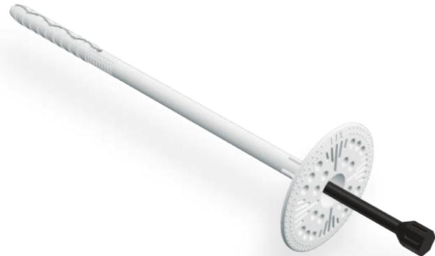
Advanced hammer-in facade plug with a polyamide pin for fixing external thermal insulation ETICS in concrete and masonry.
