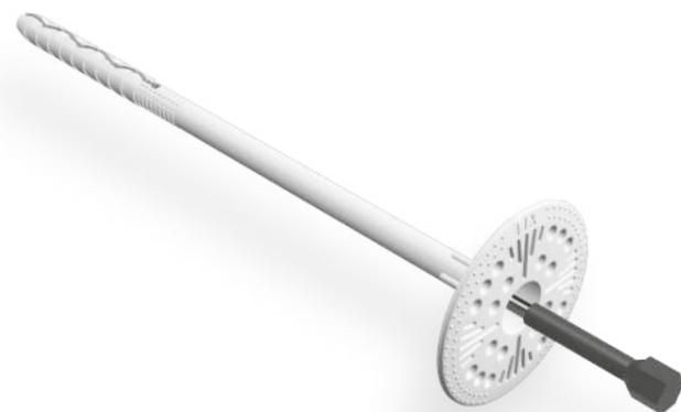
Advanced hammer-in facade plug with a metal, plastic covered pin for fixing external thermal insulation ETICS in concrete and masonry.
