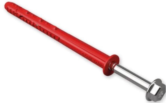
Universal frame plug with a flange and a galvanized hexagonal head screw SW10 with a TX30 socket for through-mounting.
