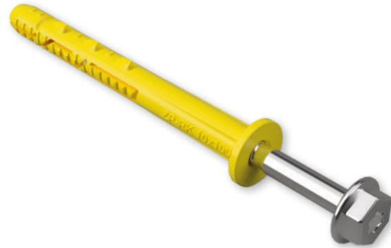
Universal frame plug with a flange and a galvanized hexagonal head screw SW13 with a TX40 socket for through-mounting.
